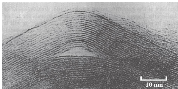
FIGURE 6.6 Transmission electron micrograph of halloysite showing lines, corresponding to basal unit layers, repeating at distances of approximately 7.2 \text{\AA} (0.72 nm). (From Clays and Clay Minerals by Sudo, T., and H. Yotsumoto. Copyright 1977 by The Clay Minerals Society. Reproduced with permission of The Clay Minerals Society in the format other book via Copyright Clearance Center.)
